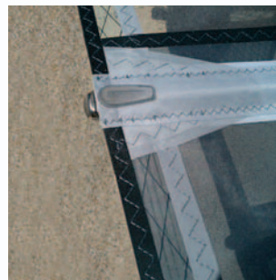
4. PU moulded batten end chafe protectors.
