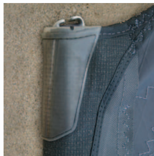
3. Mast tip chafe protector and 3D moulded head fairings.
